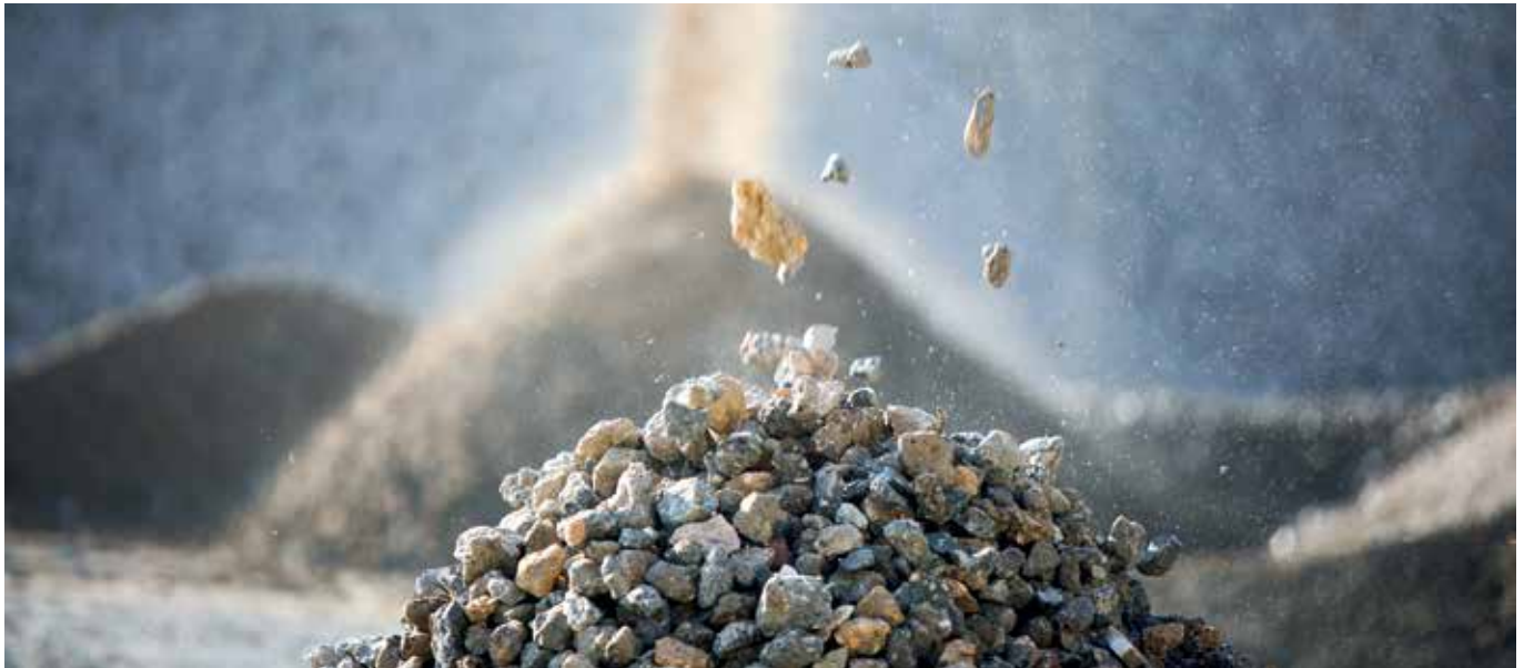
The Recycling Center Himberg makes a circular economy possible. This recycling plant produces recycled construction materials from mineral construction waste – especially asphalt, concrete, construction waste and natural rock.
